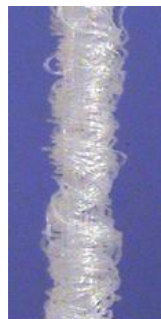
Figure 24 : Photo fil double guipé (26)
