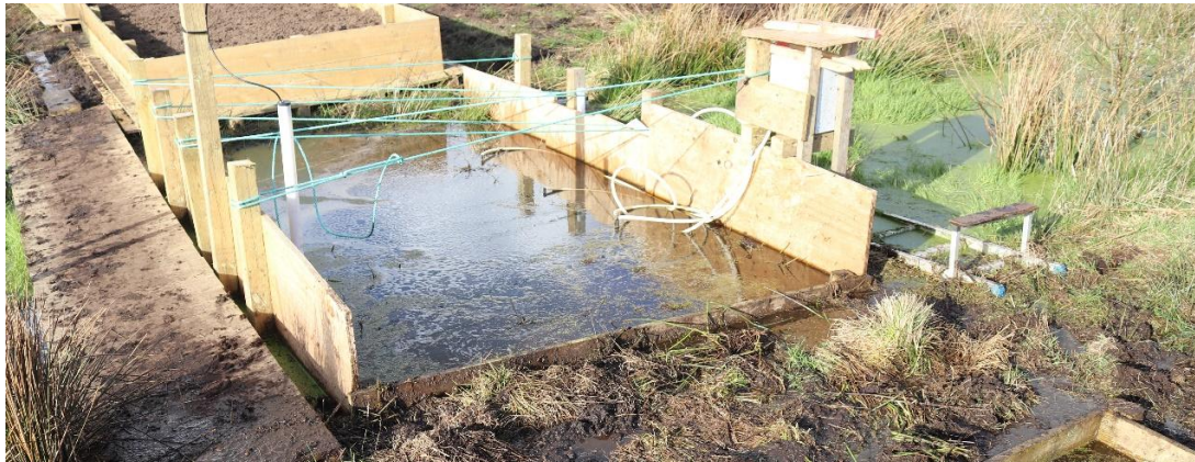
Figure 5 : Treatment n°3 (Sky 3) ; the ditch partly was filled with the topsoil from Sky 4. Wooden plates were settled to fix the shape of this plot.
