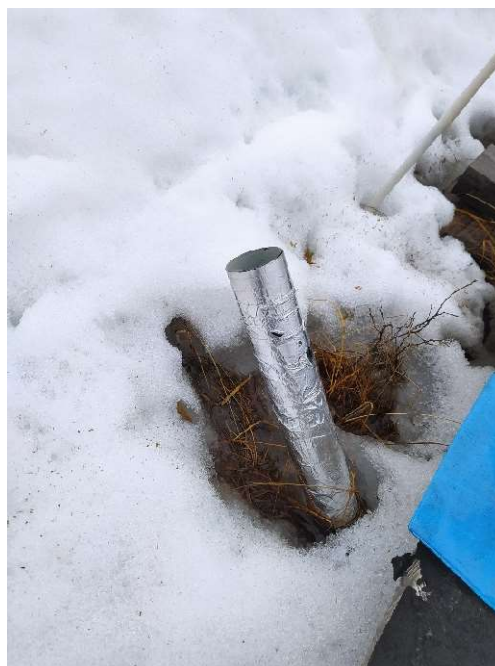
Figure 3 : Photo of the tube in the soil to scan the roots (credit : J. Helson, 2024)
