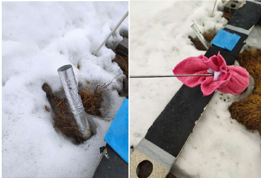
Figure 9 : Photos of the equipment used to scan the roots (left) and to clean the tube (right) (credit : J. Helson, 2024)
