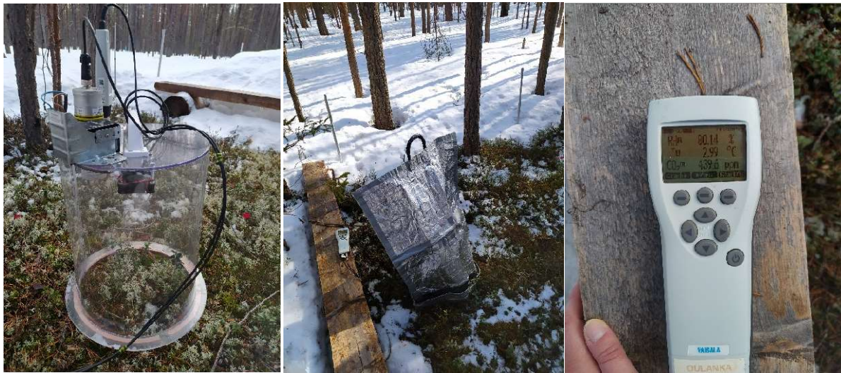
Figure 8 : Photo of the chamber and the Vaisala GMP373 instrument (credit : J. Helson, 2024)
