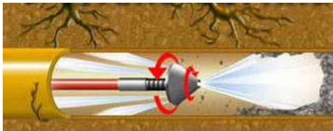
Figure 40 : Hydrocurage (Source : Normao Assainissement)
