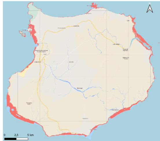
Figure 26: Boa Vista zones impacted by coastal floods (2100-1.10m)
