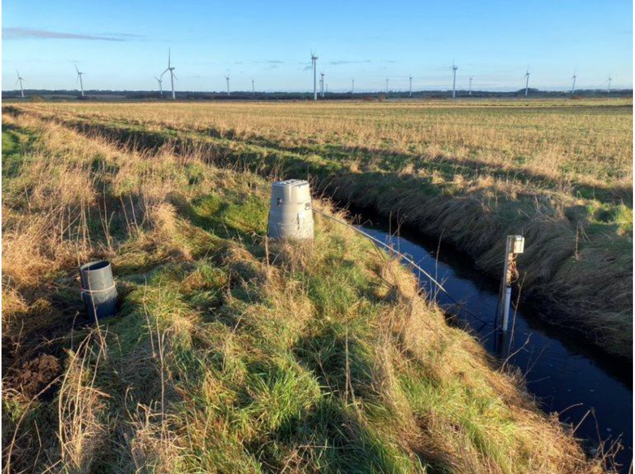
Figure 4: ISCO sampler and water level logger
