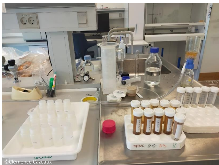
Figure 12 - Filtration of the iron samples (left) and dilution of the iron samples (right)
