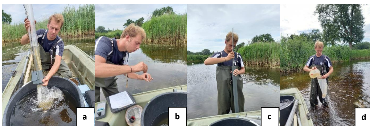
Figure 12 : a) Collection of a depth integrated water sample using a tube sampler b) Estimation of CHLa and PC concentrations using a portable fluorometer c) Determination of the water transparency using a Sneller tube d) Quantitative sampling of zooplankton (Source : Robby Wijns)
