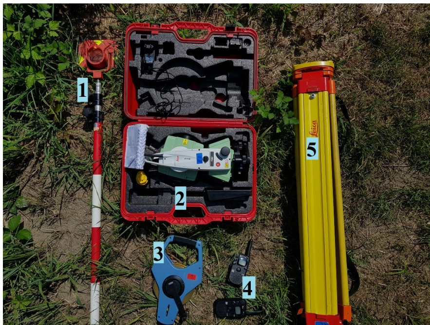
Figure 10: Topographic survey material. 1- Reflector stick. 2- Total station. 3-Measuring tape. 4- Walkie-talkie. 5- Tripod
