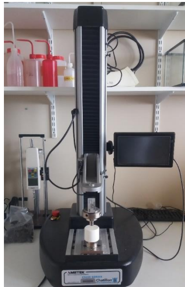
Figure 4. Dynamometer AMETEK Test and Calibration Instruments, CS225 SERIES, Chatillon Force Measurement Source : Alexandre Fouache (2021)
