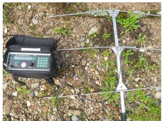
Figure 10 : R410 scanning receiver and Yagi antenna. Source : Universidade de Évora. 2015. Habitat restoration for diadromous fish in river Mondego, Portugal. http://www.rhpdm.uevora.pt/gallery.html
