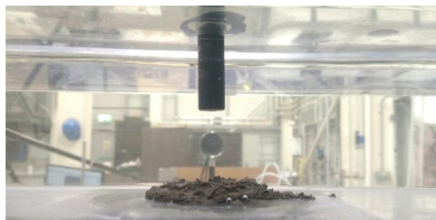
Figure 1: Erosion of a cohesive sediment core in the flume
