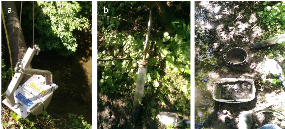
Figure 4a: Grab. 4b: Core. 4c: Cohesive sediment collected with bucket and shovel
