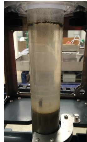
Figure 2: Core tube filled with sediment
