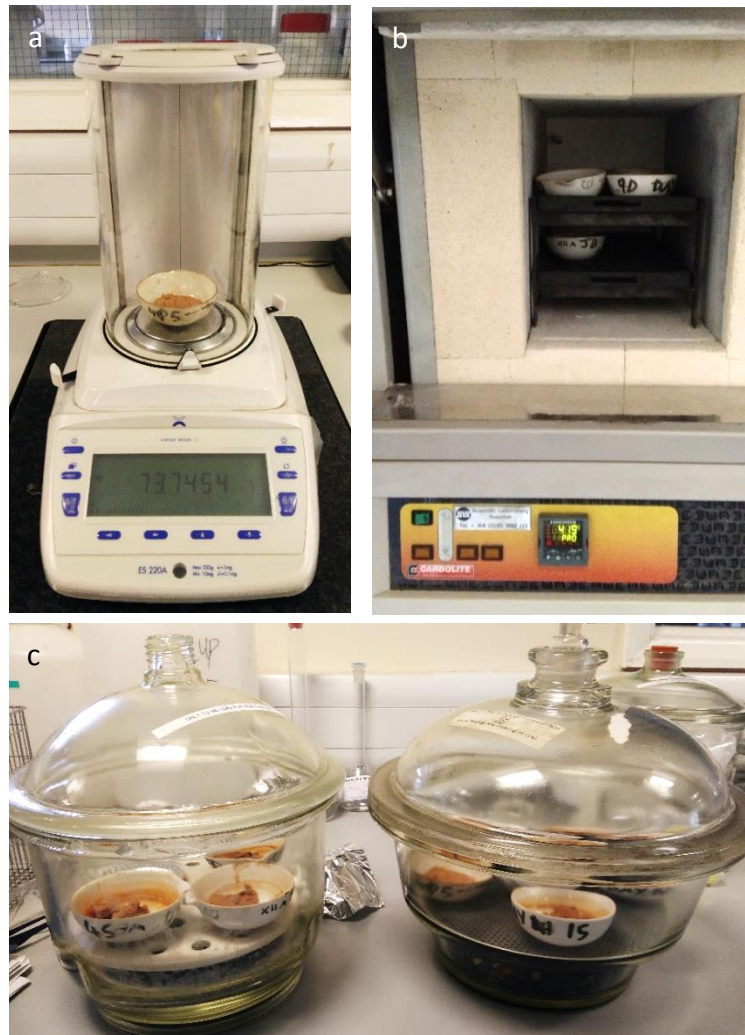
Figure 22a: Weighing of samples after ignition. 21b: Samples in the furnace at 450°C. 21c: Samples to cool in desiccators.
