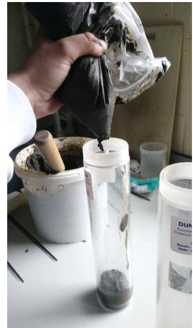
Figure 20: Filling core tube with a pipping bag
