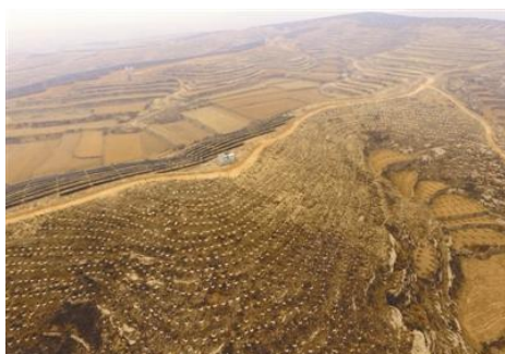
Figure 18 :Fish-scale pits of afforestation programme in Xingtai county, Hebei Province, China ( http://www.xtrb.cn/news/2016-03/23/content_536613.html )
