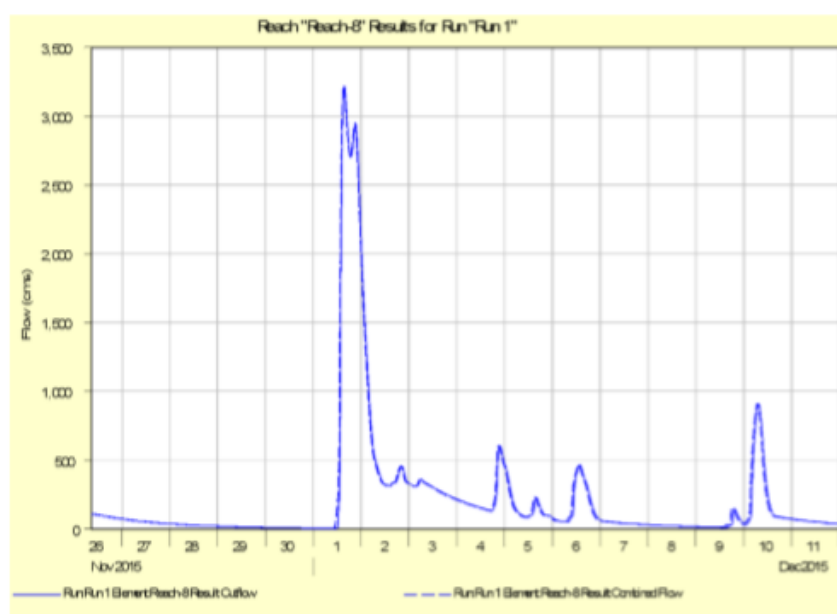
Figure 22 Floods runoff predictions using HEC-HMS for the catchment uncontrolled by Chembarambakkam tank
