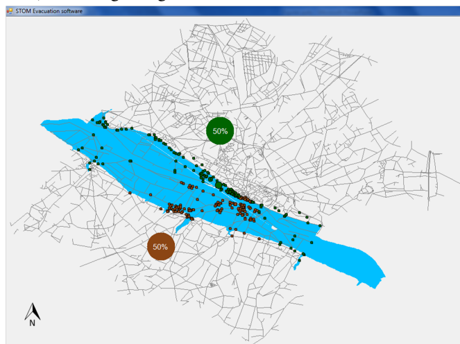
b: Assignment of buildings to safety points
