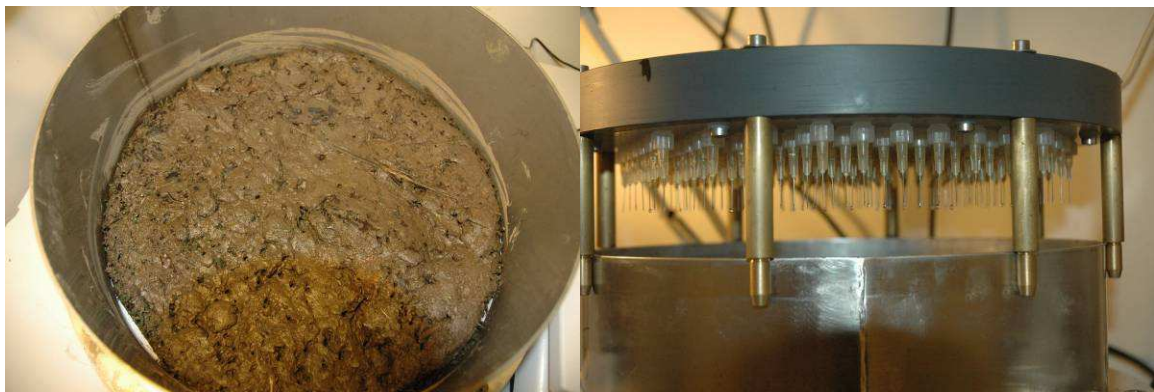
Figure 8: Cylinder with the sediment (left), upper part of the system with the needles (right)
